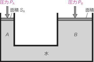
$\frac{\text{圧力 } P_A}{\text{面積 } S_A} = \frac{\text{圧力 } P_B}{\text{面積 } S_B}$ |
